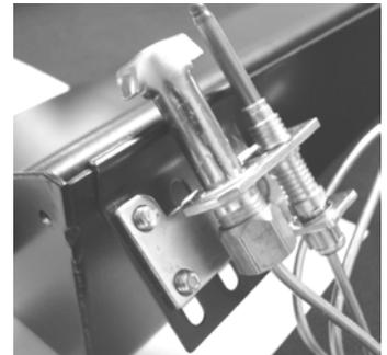
Again, being very careful, bring the copper conduit around from the thermocouple to the port on the back end of part 1 and connect it.
